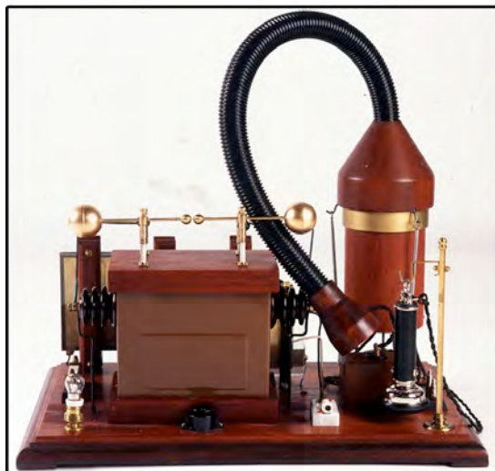
Figure 2. Replica of Landell's Wave Transmitter . It was assembled and tested (May 23rd, 2004) by Marco A. C. Moura, a researcher from Porto Alegre (photo courtesy of M. A. C. Moura – Porto Alegre, Brazil). On the left side the Ruhmkorff coil and the metallic spheres (spark-gap generator) could be seen. In the right side there is the phonetic switch (tube and resonant chamber).
